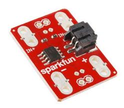
**Description:** MOSFETs are awesome. They're like a switch that you flip electronically! This SparkFun MOSFET Power Controller makes it easy to switch a battery supply on and off using your favorite microcontroller. The board also has sewable pads so you can use it in e-textile projects that need more juice.
